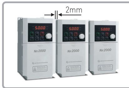
Side-by-Side Installation (2mm between drives)
